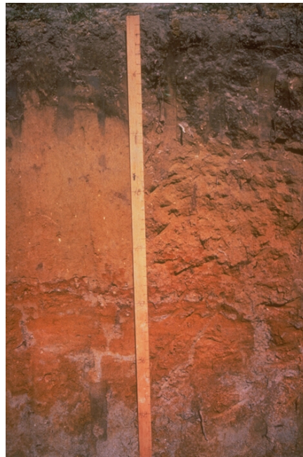
Figure 26. This is a moderately well drained soil with redoximorphic features occurring starting at 0.75 m (30 in.)
