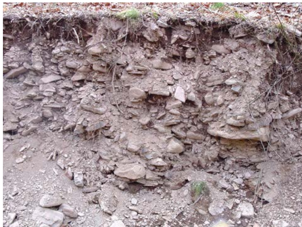
Figure 19. This soil profile contains cobble size rock fragments in a high enough concentration to put an extremely cobbly modifier on the texture.
