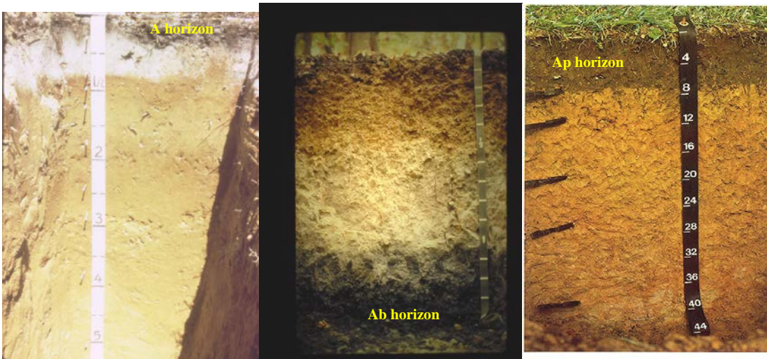
Figure 7. The soil profile to the right shows a well drained soil with an A horizon from the surface to a depth of 5 cm (2 in.). The measuring tape is in feet. The middle soil profile is a somewhat poorly drained soil with the top of the gray due to wetness occurring at 40 cm (16 in.). Tape measure is in meters. The middle soil profile has a buried A horizon starting at 1 m (40 in.). The soil profile to the left is moderately well drained with an Ap horizon from the surface to 20 cm (8 in.).
