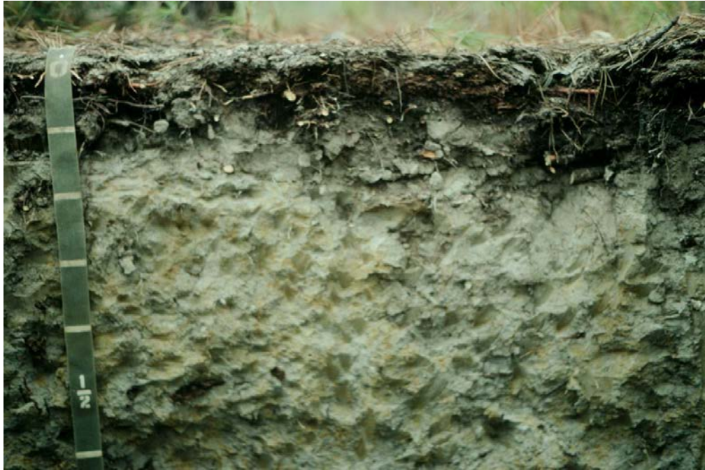
Figure 14. This soil profile is a hydric soil. The predominance of gray colors with splotches of red near the soil surface demonstrates the typical pattern of redoximorphic features found in a hydric soil.
