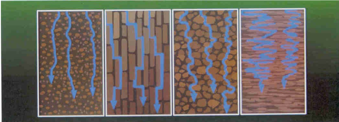
Figure 21. Paths of water flow through soils with granular, prismatic, subangular blocky, and platy structure, respectively
